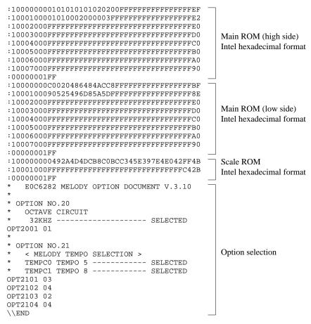
Note End mark "¥¥END" may be used instead of "\\END" depending on the PC used. (Because the code of both \ and ¥ is 5CH.)
